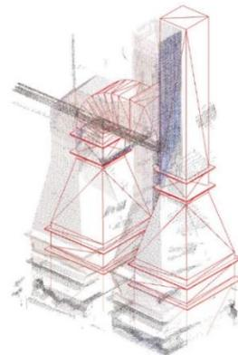
Figure 6.4: Point cloud compared with red wireframe of construction model
