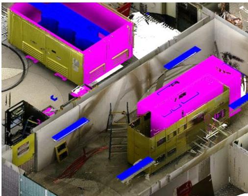
Figure 6.3: Coloured point cloud compared to model (magenta and blue elements)
